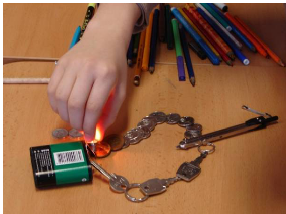
Figure 3. Non-traditional electric circuit
