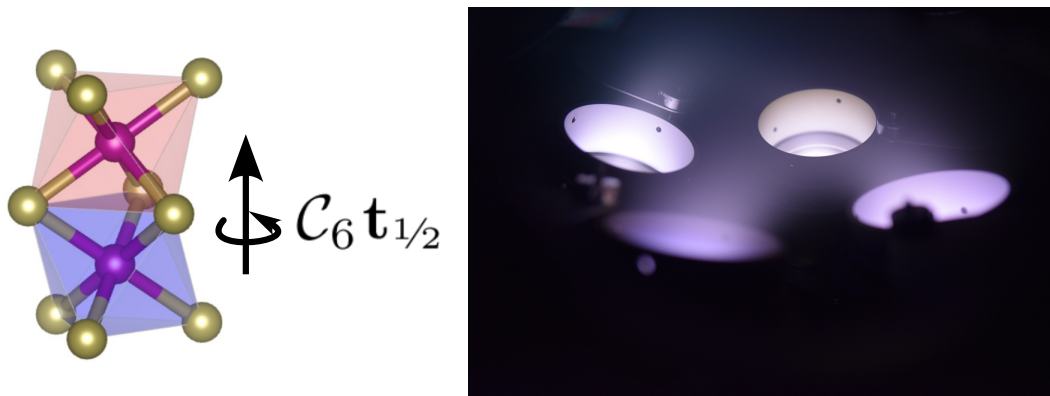
Figure 1: (left) Sketch of the unit cell of an altermagnetic material with two opposite magnetic sublattices indicated by blue and red environment linked by rotational symmetry operation. (right) Photograph of plasma in a magnetron sputter deposition system.
