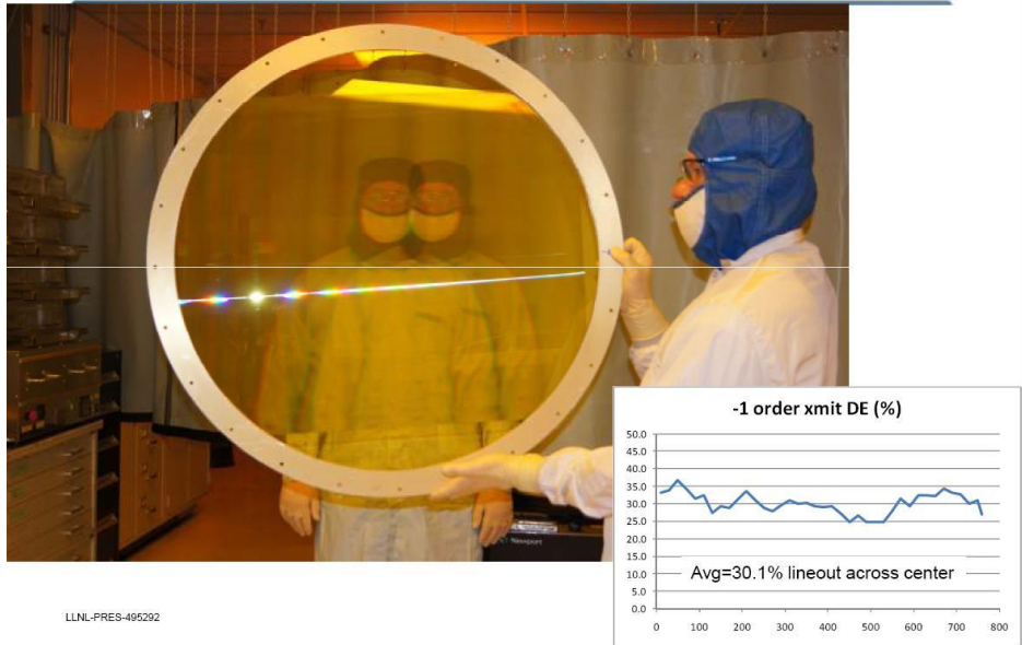
Figure 12 – Thin film replicated optics from DARPA MOIRE Ball-LLNL program. The thin (~ 30 micron) plastic film is replicated from an etched mandrel. Areal mass of the film is approximately 60 g/m 2 with actual optical mass dominated by mounting ring and not the optic itself. Thin glass and other materials are other possibilities for these lightweight replicated optics. In our system all optical elements are identical leading to mass production replicated techniques being optimal. Credit: DARPA.
